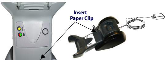
Figure 5. Disconnecting the Cable
