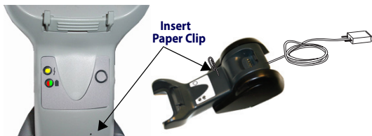
Figure 8. Disconnecting the Cable
