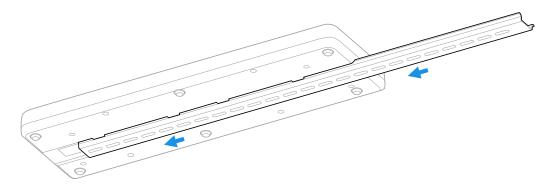
2. Secure the DIN rail to the flat surface with the hardware.
